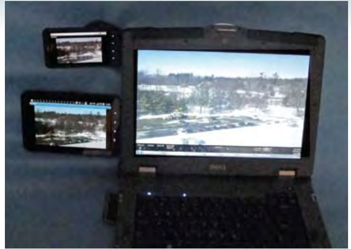
A live image stream from OAI's KJ-640 gimbaled sensor is highlighted by having the live transport stream simultaneously displayed on a ruggedized laptop, a Galaxy tablet and a Droid X phone. Photo courtesy OAI.
